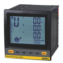
Celex Smart Power Meter PA Series is a multimeter that carry out extended ranges of measuring, monitoring and analysis of various types of electric parameters. Designed with the advanced built-in LoRaWAN wireless transceiver module, the measured power data is collected and uploaded to Celex cloud server for both real-time and historical analysis.
