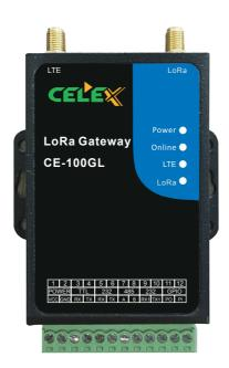
Celex Smart Gateway CE100GL is designed based on a LoRa to 4G wireless data transmission gateway, which is capable of transmitting the data to the Cloud for Al analysis and storage. Acting as a bridge between the cloud platform and the terminal module or target devices, Celex Smart Gateway CE100GL is indeed the most suitable choice for users who see to IoT application scenarios with low power consumption, medium data amount as well as long distance communication.
